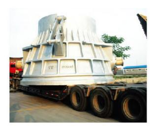
Slag pot is widely used in steel and casting industry. It is a kind of container that takes up steel slag. The slag pot can be divided into three parts, slag body, trunnion and turning mechanism.
